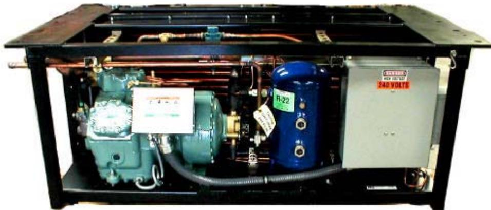
Units are available with several different sizes of compressor available, depending on the performance required for a particular passenger car. Depending on the compressor and fan size, units range from 7.5 to 10 tons of cooling capacity.
