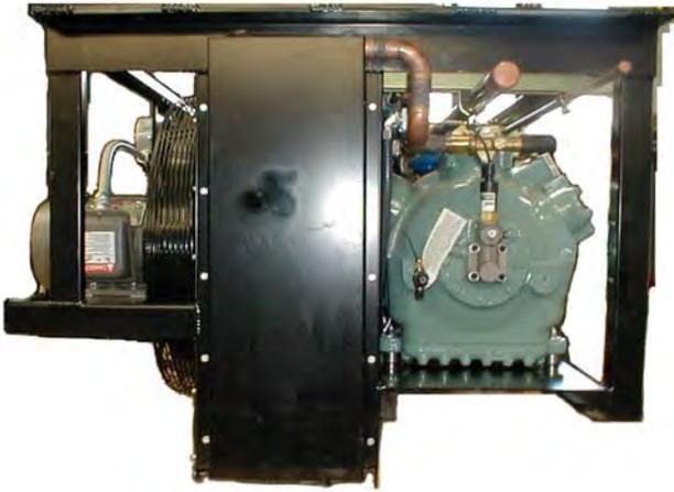
As mentioned above, Northwest Rail Electric condensers are specifically designed for mounting under a railroad passenger car. The shape of the frame allows the side of the unit that faces the side of the car to have the most clearance. Mounting angles at each end of the frame are designed for a supporting frame, so that railroad policies about supporting under-car mounted equipment with a frame structure may be easily followed.
