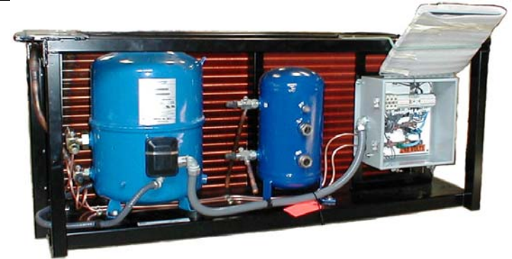
Air Conditioning Condensers designed for Under-Car Mounting, Copper Coils for Best Survival in Railroad Environment, and Wide Fin Spacing for Easier Cleaning. NOT A MODIFIED building unit!
