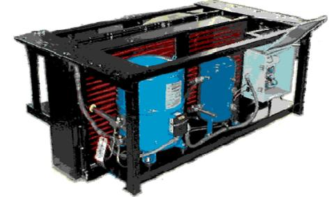
Our standard evaporator unit (**above, left**) includes blowers, heater and air conditioning evaporator that will fit in most retrofit applications. Our standard condenser (**above, right**) is built to fit most passenger cars as well. All components are constructed with railroad service in mind. For example, the condenser coil features widely spaced copper fins, so the unit will survive under-car dirt and resulting cleaning. Powder coat finish assures metal parts a long life.
